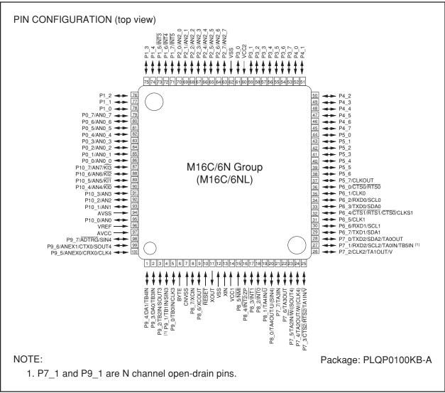
Figure 1.3 Pin Configuration (Top View) (1)
